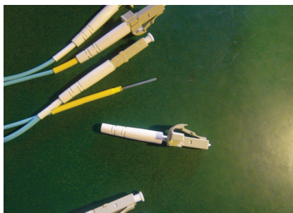
Figure 6: Failed Cable Pull and Cable Flex Tests for MPO/MTP-to-LC Hybrid Assemblies
