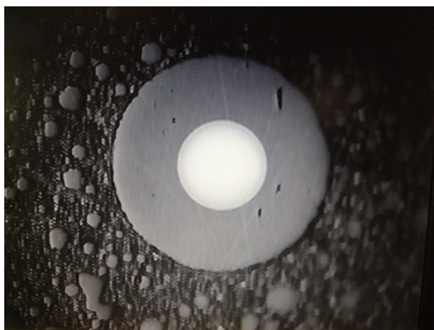
Figure 3: End face Contamination and Surface Defects for MPO/MTP Trunk Assemblies (Note: One fiber end face shown for clarity)
