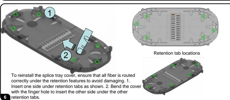
Trays can be stacked to match enclosure fiber capacity.
