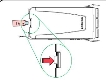
To remove the top cover, push in the rear release latch as shown.
