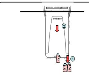
To remove the cassette from the rear of its mounting position, pull the tether while lightly holding the cassette.
