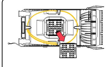
If using the 24-fiber version of the splice cassette it will be necessary to remove the top-level splice sleeve holder. Pull it up and it will detach from the bottom splice sleeve holder.
