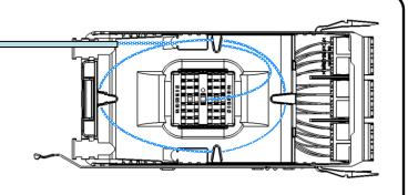
Prepare approximately 20 in. (51 cm) of fiber length from the distribution fiber jacket for proper routing into the fiber guides as shown.
