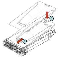
Place the cover back in place on the cassette being careful not to pinch fibers between the cassette and cover when snapping into place. Follow instructions from LightVerse enclosures and panels to install the cassettes.
