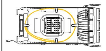
A 17 in. (43 cm) storage loop of fiber is stored in the management tray as shown. The coiled fiber should place the splice end at the splice sleeve holder. Pigtails are labeled **1** for ports 1-12, **2** for ports 13-24.
