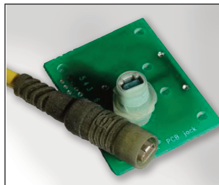
Figure 5: Ruggedized Single-Pair Connector Variant Selected by ISO/IEC for Light and Heavy Industrial Spaces
